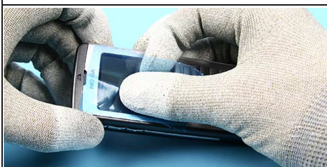
27.) Protect the window with a plastic film.
