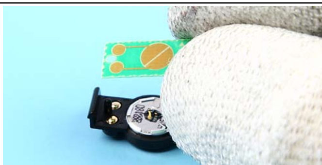
6.) Place the Earpiece Contact PWB.
