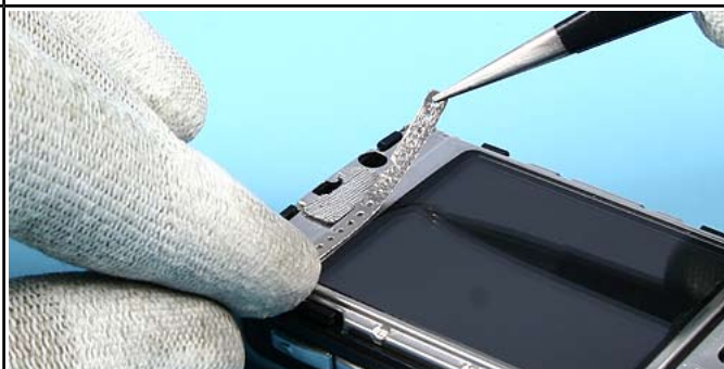
24.) Glue the Grounding Foam onto the Display Shield.
