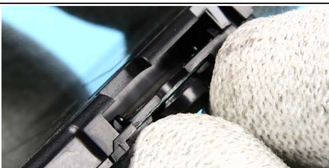
8.) Fix the Earpiece guide at the Antenna Module Assy.
