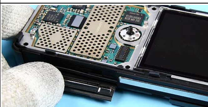
12.) Open the MMC Door before continuing.
