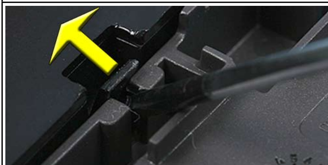
21.) Unlock the clip of the Antenna Module Assy in shown direction.
