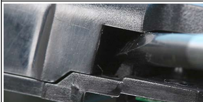
23.) Unlock both clips as shown to release the Earpiece Cover.
