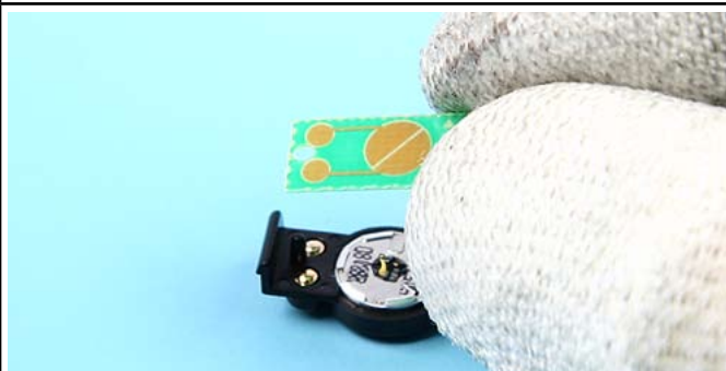
24.) Remove the Earpiece Contact PWB.
