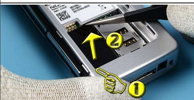
28.) Glue the MMC READER LABEL onto the MMC reader.
