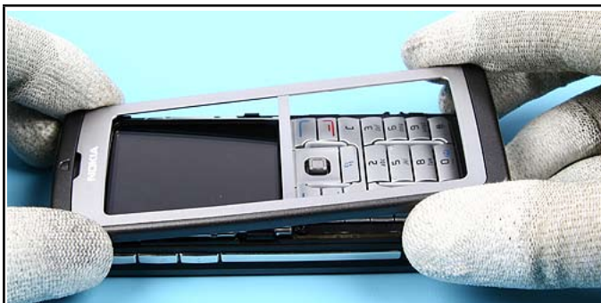
25.) Place the A-COVER beginning from the top.
