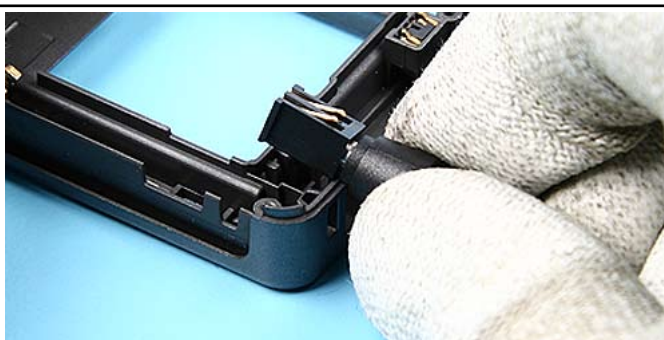
28.) Remove the DC Jack with the DC Plug.
