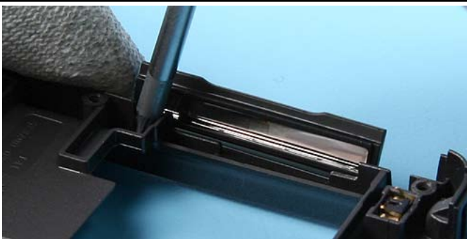
4.) Inset the MMC Door and fix it into its compartment.
