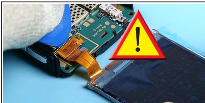
17.) Open the flex connector.
