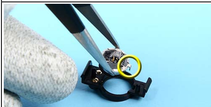
5.) Place the Earpiece, mind the guiding. Always fit a new Earpiece Adhesive when replacing the Earpiece.
